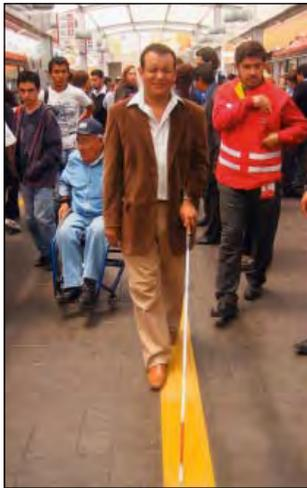
improvements include a deeply grooved tactile guideway to assist blind passengers (photo at left) and Braille information plates. Wheelchair users can access a button to operate a warning light to notify approaching bus drivers to carefully dock their buses to reduce the horizontal gap of some 10 cm between the raised station platform and the floor of the bus.
