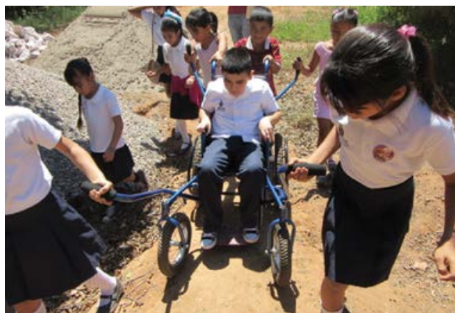
Photo above shows an all-terrain “spider” wheelchair built to get a child to school over rough terrain in rural Mexico. The projections enable other children to help push and pull the wheelchair. - Photo by permission of HealthWrights
