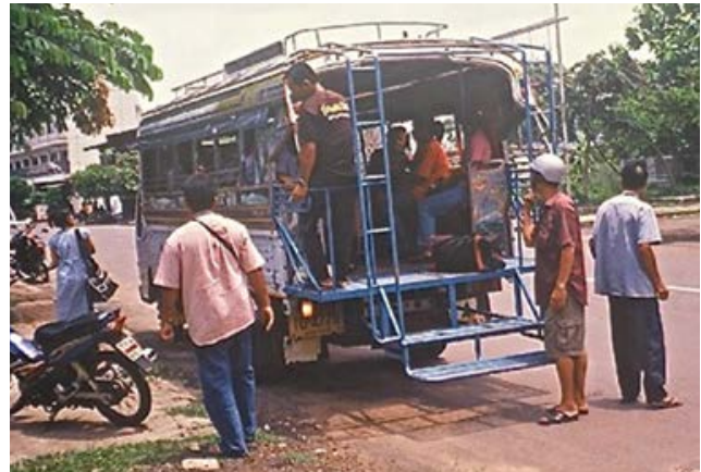
This bus in Cuba is high floored for rural use, with slanted stairs and fairly adequate hand rails to provide relatively better access than in the absence of such features. A wide variety of passenger cabins modified to fit on different truck bodies are used in many countries. Though clearly not accessible to those persons with disabilities who must remain in wheelchairs during travel, in many countries people of good will tend to be more “hands on” in assisting persons with disabilities. Standards of accessibility taken for granted in some countries are less observed or ignored in others. - Photo by CGB “Kit” Mitchell
